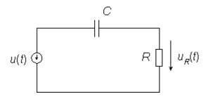
Above a simple network consisting of an ideal voltage source, a linear time-invariant resistor and a linear time-invariant capacitor is given.
